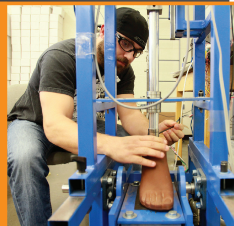
Graduate student Joshua Bowen tests the durability of a prosthetic foot in the LIMBS International laboratory. The focus of the lab and nonprofit organization is to create highly functional, ultra-low-cost prosthetics for the "poorest of the poor." Photo by J.R. Hernandez
